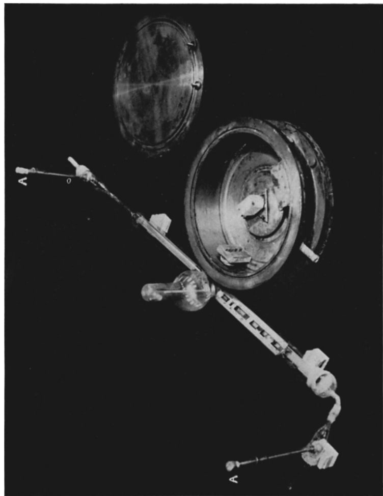
PLATE 4.1. H. G. J. Moseley's X-ray spectrograph, from experiments with which it became clear that the atomic number of an element is numerically equal to the positive charge on the nucleus.
